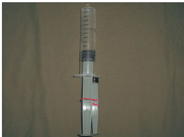
Figure 4: The big loop is used to anchor the 5cc piston as a stopper
