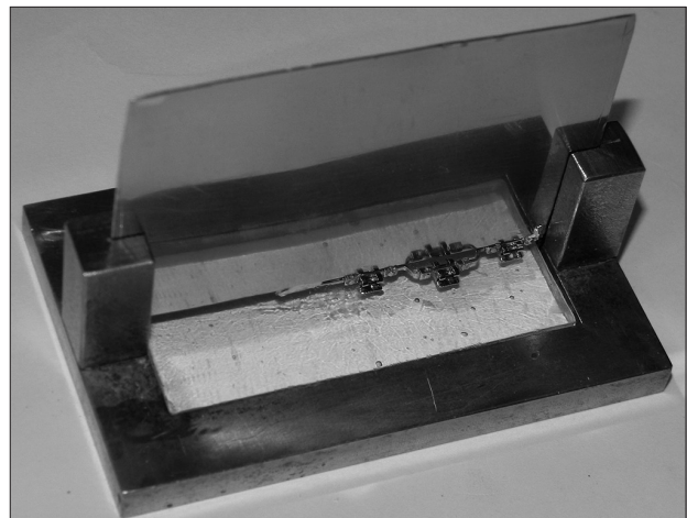
Figure 1: Device used to standardize the bonding procedure
