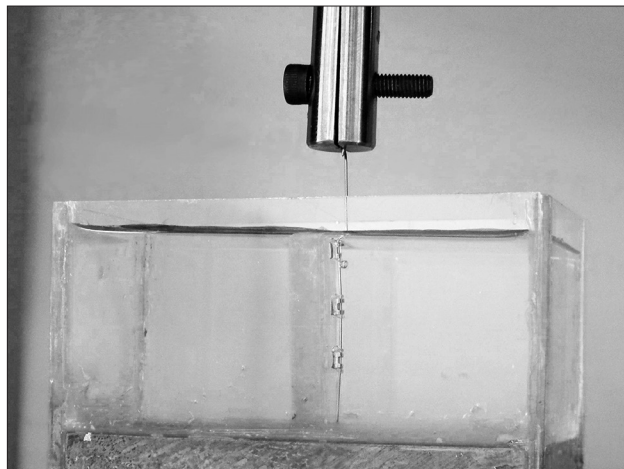
Figure 2: Device used in frictional force test
