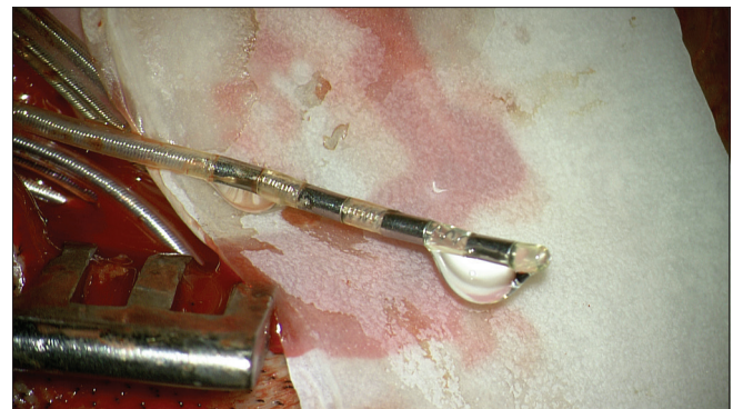
Figure 2: A photograph showing cerebrospinal fluid egress from the proximal end of quadripolar deep brain stimulation electrode lead. Cerebrospinal fluid egressing from fine gaps between the metallic electrode contacts and electrode spacing was observed
