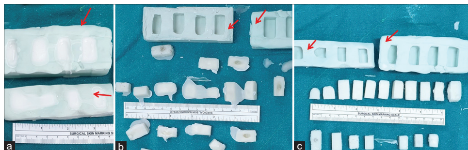
Figure 3: Shows silicone mould (red arrows) filled up with bone cement (a). Bone cement spacers removed from the moulds (b) and after removal of spilled over bone cement (c) by instruments like nibbler
