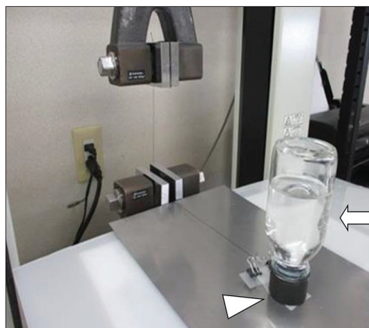
Figure 2: Friction coefficients of neurosurgical patties were measured using the friction module test system (Shimadzu Corp., Kyoto, Japan). The neurosurgical patty (arrowhead) was placed on the stainless steel board (SUS304), and one side of the patty connected to the pulling system. A 150 g-3.5 cm diameter weight (arrow) was placed on the neurosurgical patty. The neurosurgical patty was pulled at 100 mm/min tension speed a length of 150 mm and the friction forces were measured
