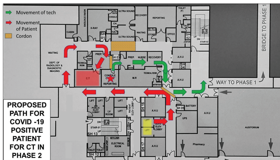
Figure 3: Plan for safe transport of known or suspected coronavirus disease 2019 patients from isolation ward. Small area painted light yellow is the elevator earmarked for patient movement from the isolation ward to the first floor computed tomography. Area painted light red is the computed tomography gantry. The red arrow marks the pathway of the patient and her attendants. The green arrows marks the pathway of the technologists coming in and out of the computed tomography console (asterisk). Cross-hatched yellow bars represent the cordon between these two pathways to avoid exposure of technologists who will be wearing moderate-risk personal protective equipment. The technologist will not enter the computed tomography gantry and will remotely adjust the computed tomography table
