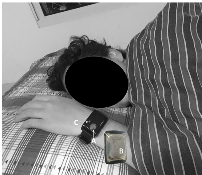
Figure 1. The circadian monitoring device, composed of an accelerometer (internal, not shown in the figure), luxometer (A), a temperature sensor (B) and event-marker button (C).
