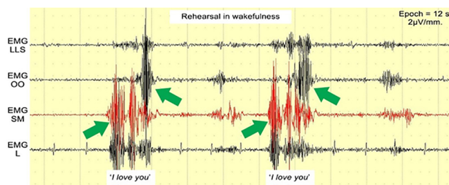
Figure 3. The “I love you” pattern in wakefulness. Abbreviations: EMG LLS = Levator labii superioris area; EMG OO = Orbicularis oris area; EMG SM = Submentalis area; EMG L = Laryngeal area.
